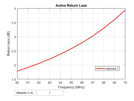
You can also view the return loss of all four elements by changing the number of elements on the plot from 1 to 1:4. See figure.
