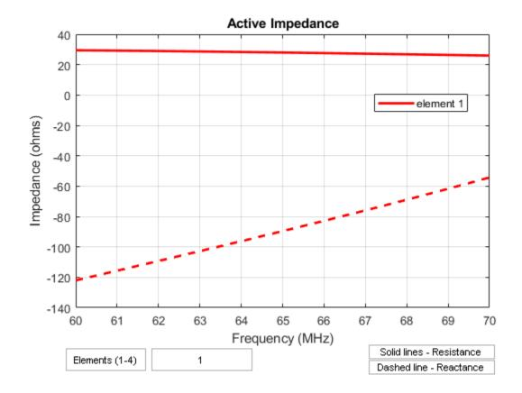
You can also view the impedance of all four elements by changing the number of elements on the plot from 1 to 1:4. See figure.
