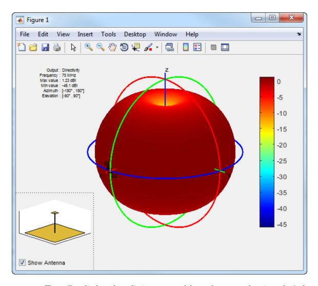
The toolbox displays the radiation pattern of the top-hat monopole using *spherical* coordinate system represented by azimuth and elevation angles.
