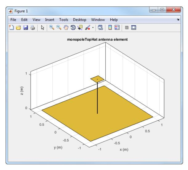
The toolbox displays the top-hat monopole antenna in the rectangular or Cartesian coordinate system.
